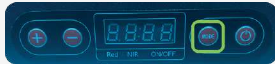
Select Mode - Red Light, Near Infrared, or Both *Power must be OFF to change Mode
