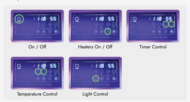
Press the key to turn light on/off. To change the color hold the key for 8 seconds. You will hear the beep and the temperature display will show "LE". Press the key to toggle between colors. Once you have the setting you want, do not touch press any buttons for 5 seconds and your setting will be saved.
