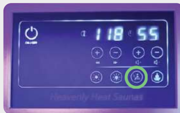
Heaters On / Off
