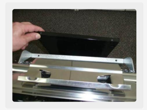
7. Screw the mounting bracket back to the black mounting plate.
