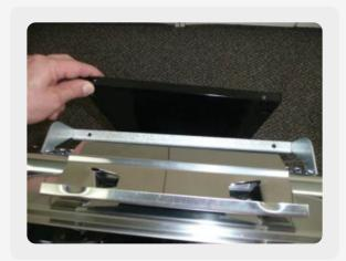
3. Remove black hanging bracket from bottom of heater.
