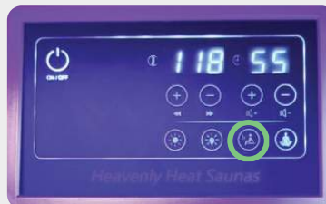
Heaters On / Off
